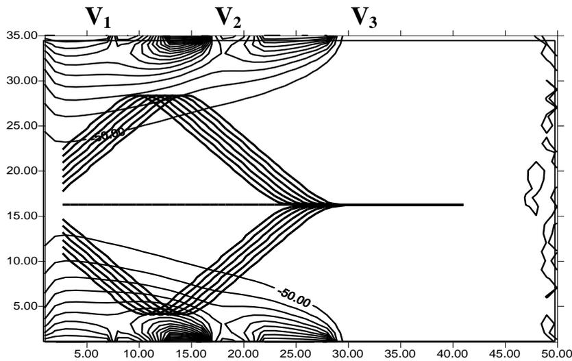
Fig (6) shows the ions beams are trundling at a distance  $V_1=V_3 = - 500$ ,  $V_2 = - 1000$
