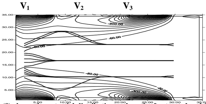
Fig (8) shows the potential distribution and path of extracted and focused ions by the electrostatic lens having three electrodes of the same size and shape when the voltage polarities are reversed  $V_1=V_3 = -1000$ ,  $V_2 = -300$
