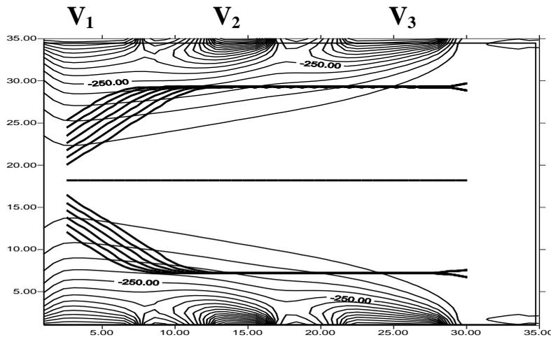
Fig (5) shows the potential distribution and path of extracted and focused ions by the electrostatic lens having three electrodes of the same size and shape  $V_1=V_3 = -700$ ,  $V_2 = -1000$
