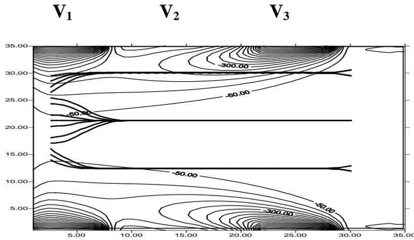
Fig (7) shows the potential distribution and path of extracted and focused ions by the electrostatic lens having three electrodes of the same size and shape when the voltage polarities are reversed  $V_1=V_3 = -1000$ ,  $V_2 = -100$
