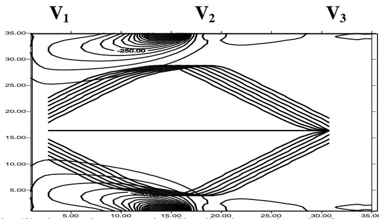
Fig (2) shows the potential distribution and path of extracted and focused ions by the electrostatic lens having three electrodes of the same size and shape  $V_1=V_3 = -100$  ,  $V_2 = -1000$
