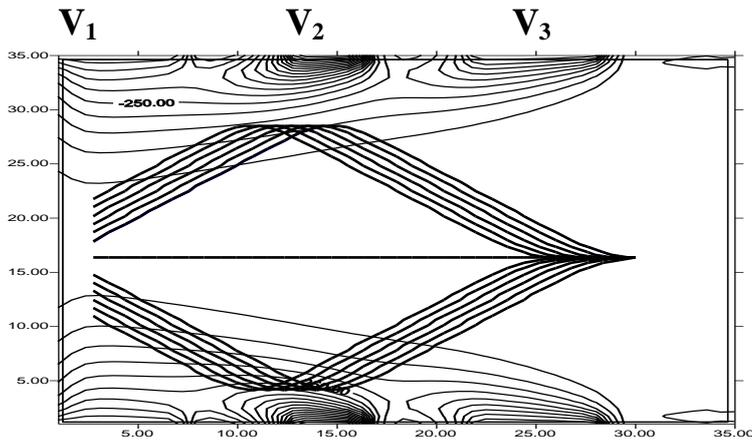
Fig (4) shows the potential distribution and path of extracted and focused ions by the electrostatic lens having three electrodes of the same size and shape  $V_1=V_3 = -500$ ,  $V_2 = -1000$
