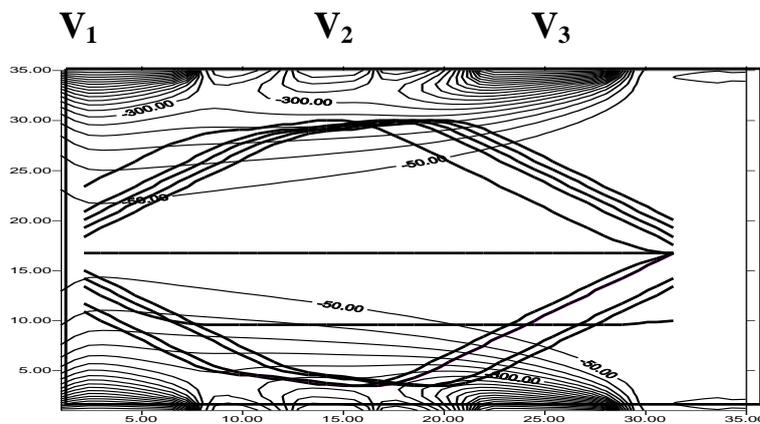
Fig (9) shows the potential distribution and path of extracted and focused ions by the electrostatic lens having three electrodes of the same size and shape when the voltage polarities are reversed  $V_1=V_3 = -1000$ ,  $V_2 = -500$
