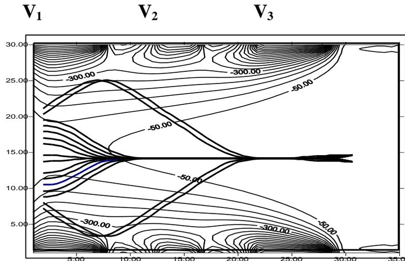
Fig (10) shows the potential distribution and path of extracted and focused ions by the electrostatic lens having three electrodes of the same size and shape when the voltage polarities are reversed  $V_1=V_3 = -1000$ ,  $V_2 = -700$
