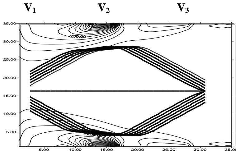
Fig (3) shows the potential distribution and path of extracted and focused ions by the electrostatic lens having three electrodes of the same size and shape  $V_1=V_3 = -200$  ,  $V_2 = -1000$
