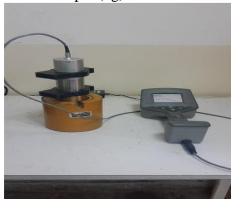
**Fig. (1):SAM940™ gamma ray spectroscopy system.**
