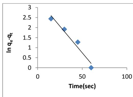
**Fig.(6) The Lagergren Model for  $Zn(NO_3)_2$  of 25 ppm at 298K Surface**
