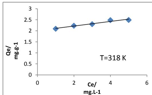
Fig.(3) The Plot of  $Q_e$  against  $C_e$  for the Adsorption a series  $Zn(NO_3)_2$  Solution at Dfferent Temperatures .
