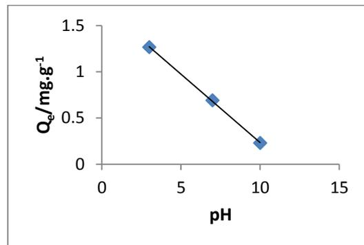
**Fig. (4)The Quantity of Adsorption at Different PH value Using Malvaparviflora at 318K for 25ppm Zn (NO<sub>3</sub>)<sub>2</sub> Solution**
