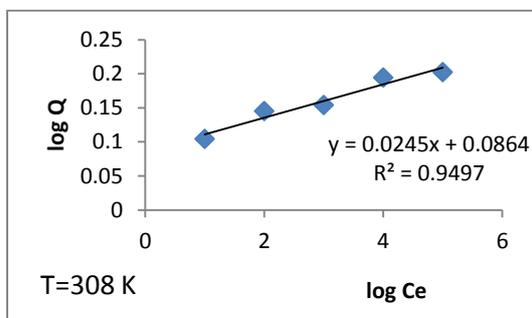
**Fig.(2) Freundlich linear Relationship between  $\log Q$  and  $\log C_e$  for a Series  $Zn(NO_3)_2$  Solution at Different Temperatures .**
