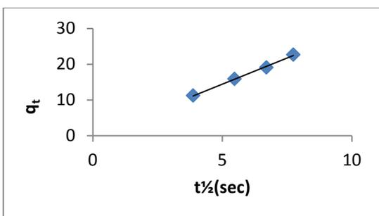
**Fig.(7) The plot of  $q_t$  against  $\sqrt{t}$  for adsorption  $Zn(NO_3)_2$  of 25ppm on malvaperviflora at 298K .**
