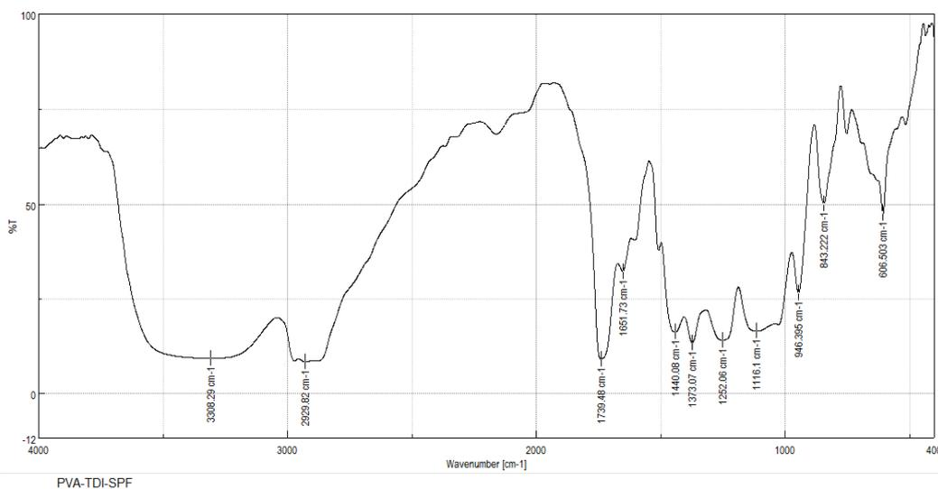
Fig.(3). FTIR Spectroscopy of PVA-TDI-SPF Mixture
