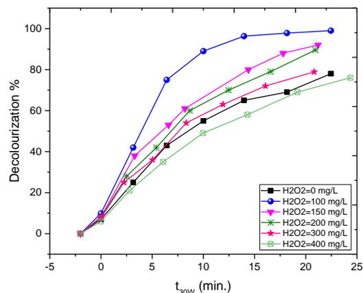
**Fig.(3). The effect of  $H_2O_2$  concentration on decolorization percent of reactive red dye**
