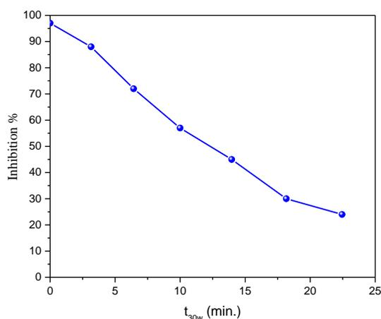
**Fig (7). Variation in inhibition percent at different reaction time for photocatalytic of reactive red dye.**
