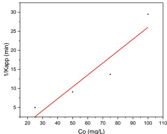
Fig (6). Variation of  $1/K_0$  vs.  $C_0$  of reactive red dye
