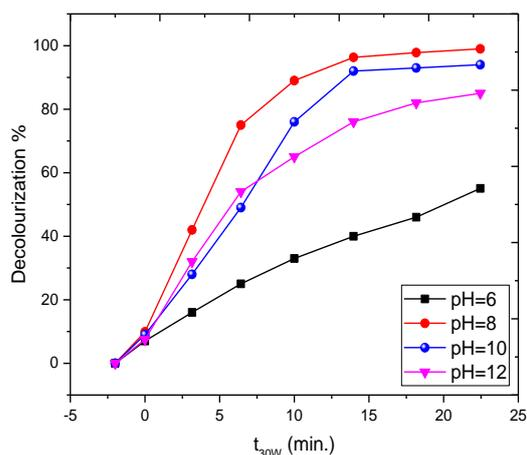
**Fig. (2). Removal efficiency of reactive red dye at different initial pH .**
