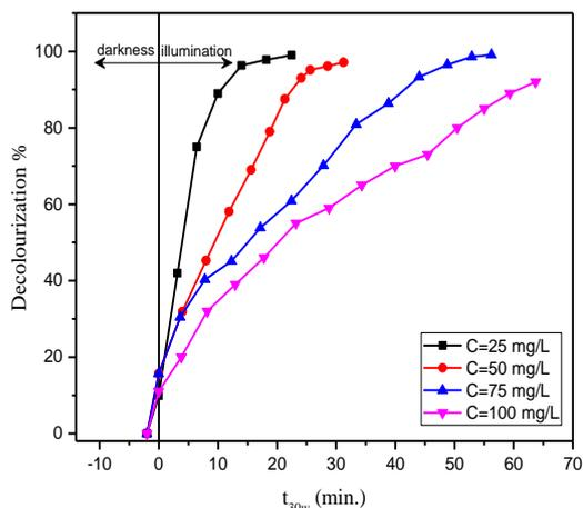
Fig.(4).The effect of initial concentration of blue dye on decolourization percent of reactive red dye.
