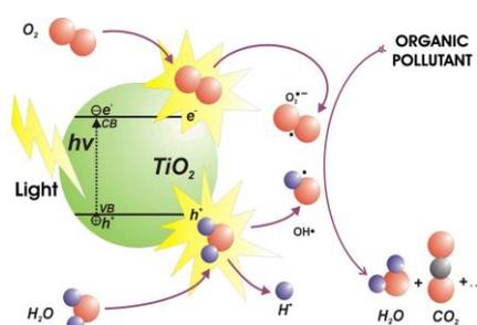
**Fig.(1). Schematic of semiconductor excitation [12].**
