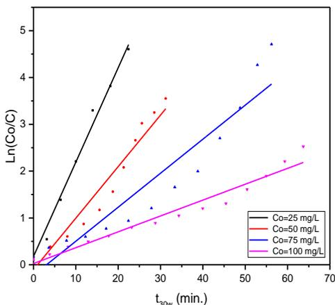
Fig.(5). The LH models for reactive red dye.
