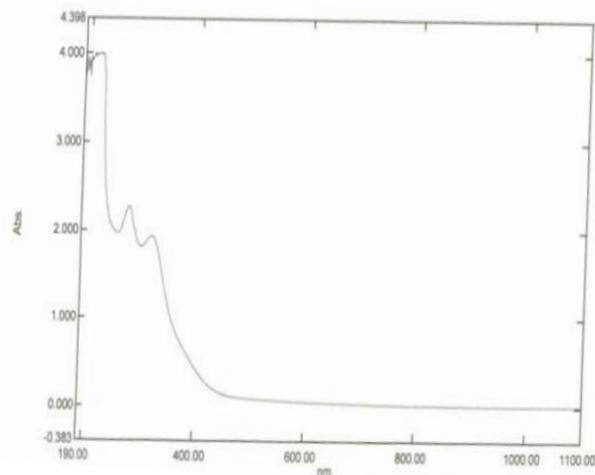
**Figure 5.** UV-vis spectrum showing absorption of ( $10^{-5} \text{M}$ ) aqueous solution of silver nitrate with *M.parviflora* extract
