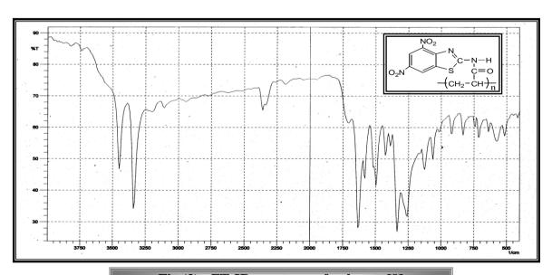
Fig.(3): FT-IR spectrum of polymer [9]
