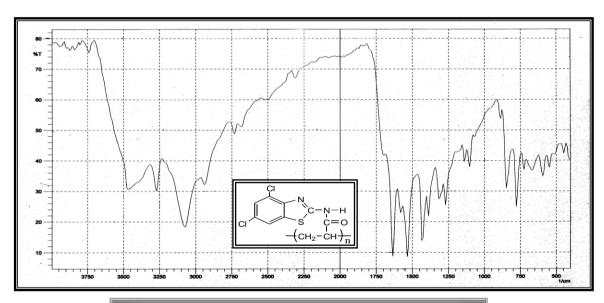
Fig. (2): FT-IR spectrum of polymer [4]
