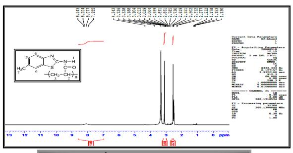
Fig. (10): <sup>1</sup>H-NMR spectrum of polymer [5]
