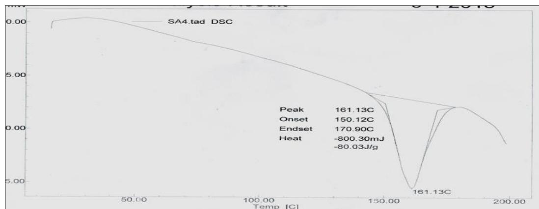
Fig.(6)DSC of Gelatin-g-methyl nadic anhydride Substitution with Salbutamol(A<sub>2</sub>)
