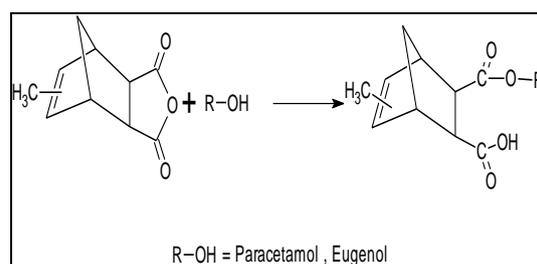
**Scheme(4) Mechanism of Ring Opening of Nadic anhydride by hydroxyl Drug**
