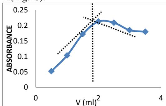
**Fig. (9): Mole ratio plot complex between Ni(II) and metformin**
