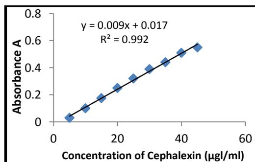
Fig. (4): Calibration Curve for Cephalosporin with  $\text{KMnO}_4$  in Alkaline Medium by Molecular Absorption Spectrophotometry.
