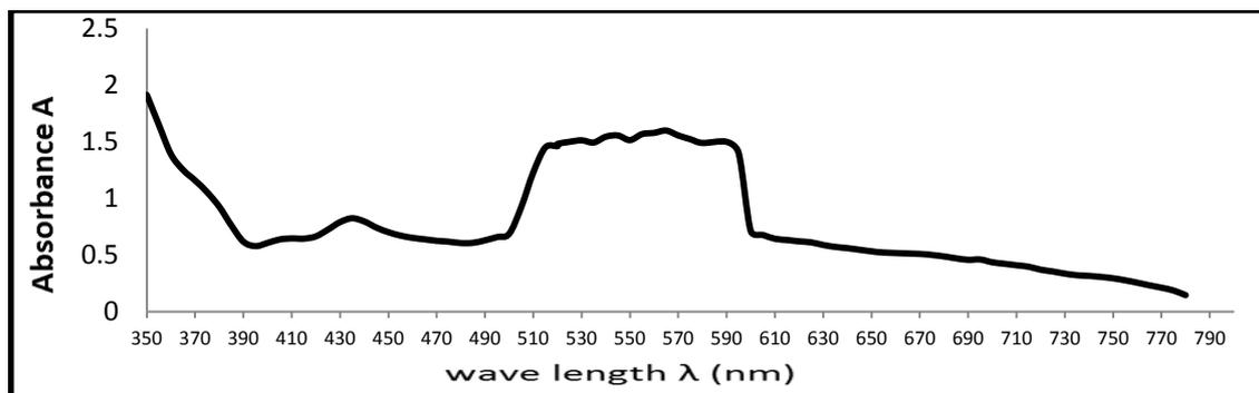
Fig. (2):Molecular Spectrum of  $\text{KMnO}_4$  in Alkaline Medium.
