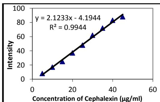
Fig. (3): Calibration Curve for Cephalosporin with  $\text{KMnO}_4$  in Alkaline Medium by Flame Atomic Emission Photometry.
