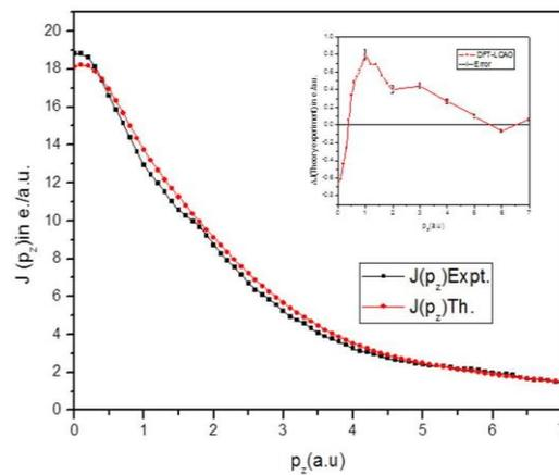
**Fig.4. The Absolute DFT-LCAO and Experimental Compton Profiles of  $\text{Cu}_2\text{Sb}$ . Inset Shows the Difference Between Two Data. Both Profiles are Convoluted with the Gaussian of 0.6 a.u. FWHM.**
