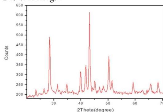
**Fig.1. XRD Patterns of Cu<sub>2</sub>Sb of Different Size**
