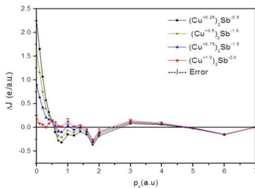
**Fig.2. Difference ( $\Delta J$ ) between Convoluted Ionic and Experimental Compton Profiles of  $\text{Cu}_2\text{Sb}$ . Experimental Errors ( $\pm\Sigma$ ) are Also Shown at Points. All Ionic Profile are Convoluted with the Gaussian of 0.6 A.U. FWHM.**
