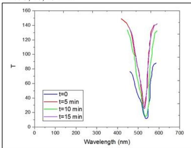
**Figure 3. Shows the transmittance of the polymer sample (PMMA) doping with Rhodamine (R3GO) before and after exposure to plasma and for different times 5, 10, 15 min.**
