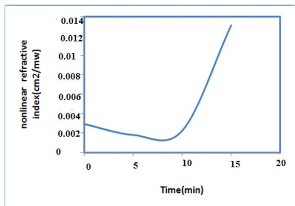
**Figure 7. Shows the relationship between the nonlinear refractive index  $n_2$  and the time of the Polymer membrane (PMMA) doping with Rhodamine (R3GO).**
