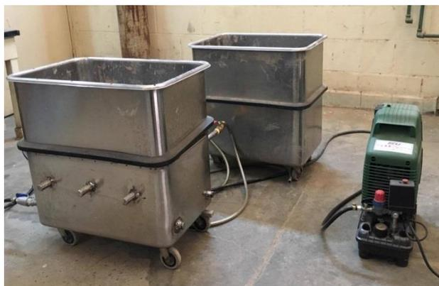
**Figure.1**The pilot-scale stainless steel tanks of Bio pile system
