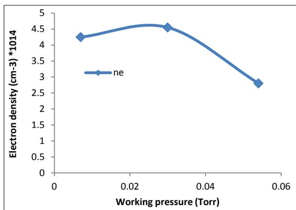
**Figure 9. Effects of varying working pressure on  $n_e$  ( $\text{cm}^{-3}$ ).**
