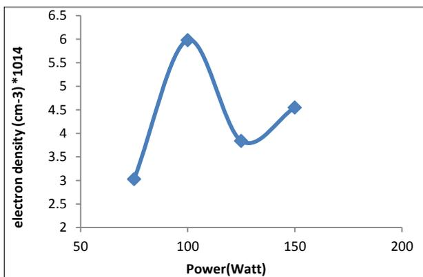
Figure 5. Effect of RF power on the electron density (cm<sup>-3</sup>)\*10<sup>14</sup>.
