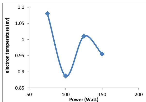
**Figure 4. Effect of RF power on the electron temperature (eV).**
