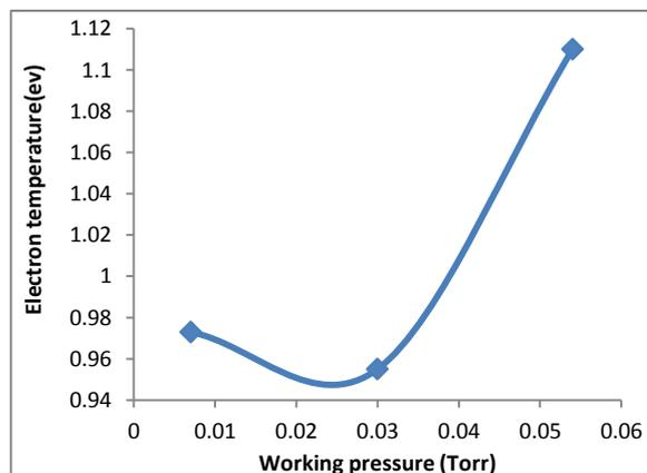
Figure 8. Effects of varying working pressure on T<sub>e</sub> (eV).
