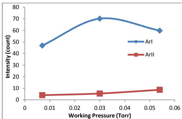
Figure 7. Effects of varying working pressure on Intensity.
