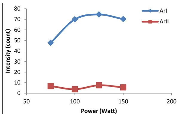
**Figure 3. Variation of ArI (750.37 nm) and ArII (434.5nm) lines intensity with RF power at  $3 \times 10^{-2}$  torr.**
