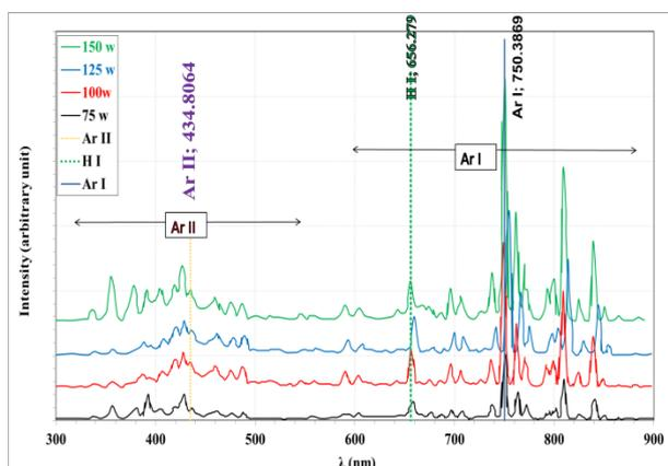
**Figure 2. The emission spectra for plasma argon at different sputtering power.**
