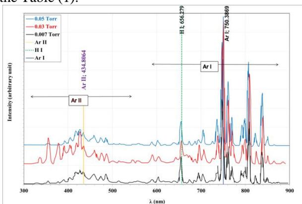
Figure 6. The emission spectra for plasma argon at different working pressures.
