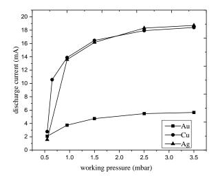
Figure4. The discharge current as a function of working pressure in argon gas discharge plasma
