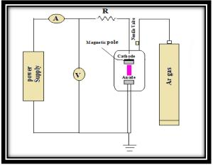
Figure 1. Experimental setup of the magnetron sputtering system
