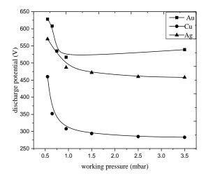
Figure 5. The discharge potential as a function of working pressure in argon gas discharge plasma
