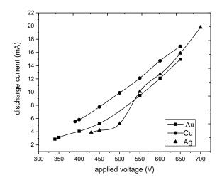
Figure 3. The discharge potential as a function applied voltage in argon gas discharge plasma
