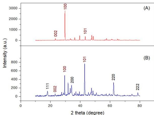
**Figure 3. XRD Pattern of the CNRS. (A) PP without catalyst at 1000 °C for one hour of pyrolysis. (B) PP with catalyst MgO at 1000 °C for one hour of pyrolysis.**
