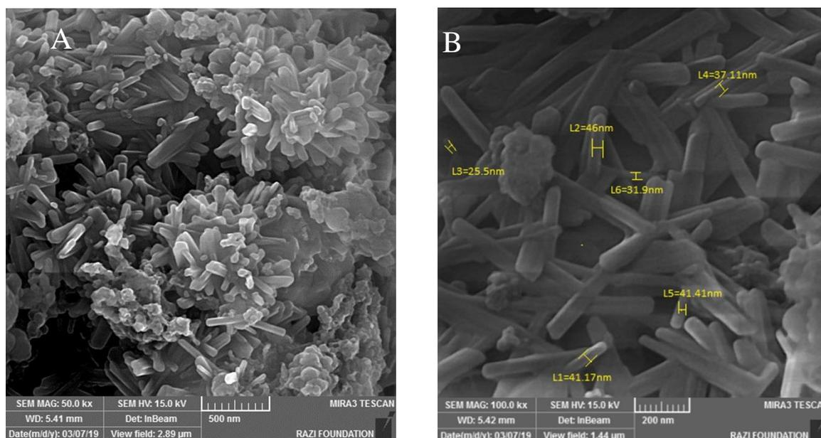
Figure 4. FESEM image of CNRs grown on MgO (A) 500nm (B) 200nm
