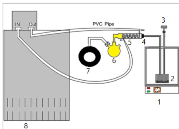
**Figure 1. Schematic diagram of unit used for synthesizing carbon nanostructures by pyrolysis method. In this diagram, 1) Electric furnace, 2) Stainless steel reactor, 3) tube nozzle containing catalyst, 4) Rubber, 5) Condenser, 6) three neck round-bottom flask, 7) Rubber bag to collect the resultant gas, 8) Water bath.**
