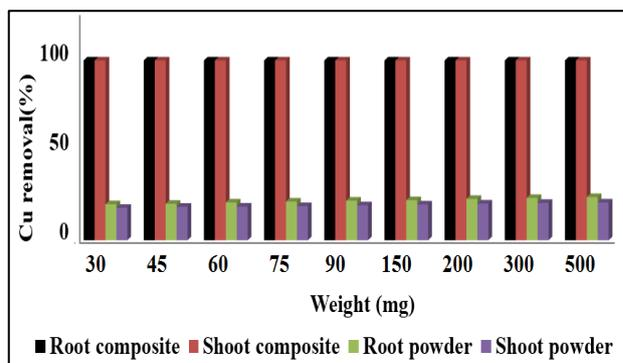
Figure 3. Removal percentage of Cu in the presence of water hyacinth parts within 24 hr and reference(0.0205 ppm).
