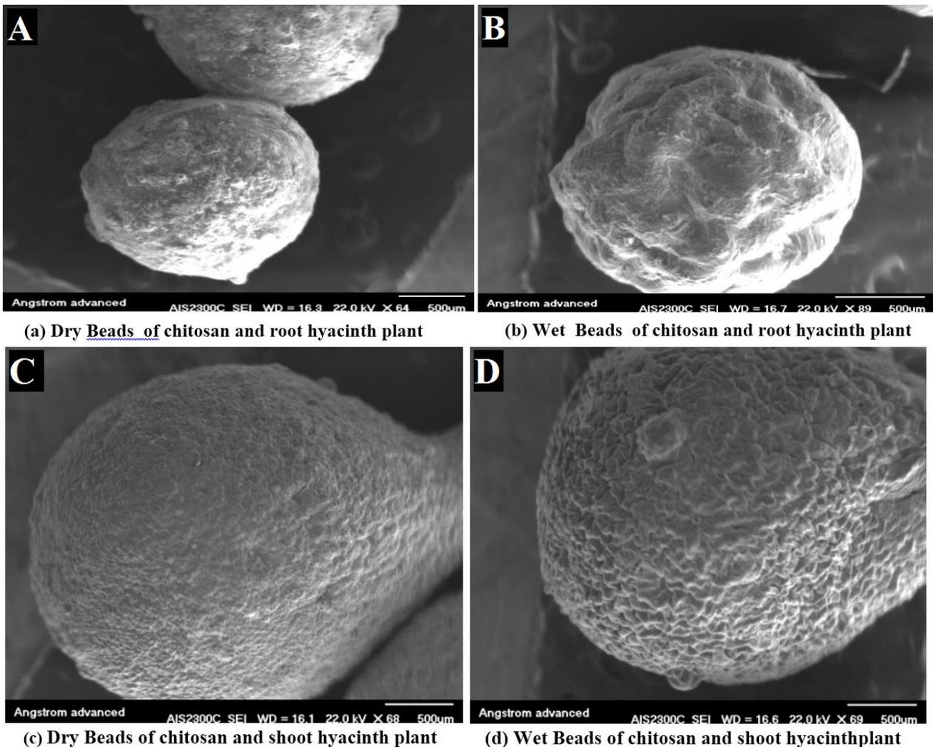
Figure 7. SEM photographs of chitosan with root and steam beads
