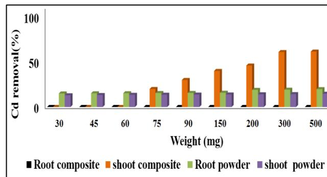
Figure 4. Removal percentage of Cd in the presence of water hyacinth parts within 24 hr and reference (0.0063 ppm).
