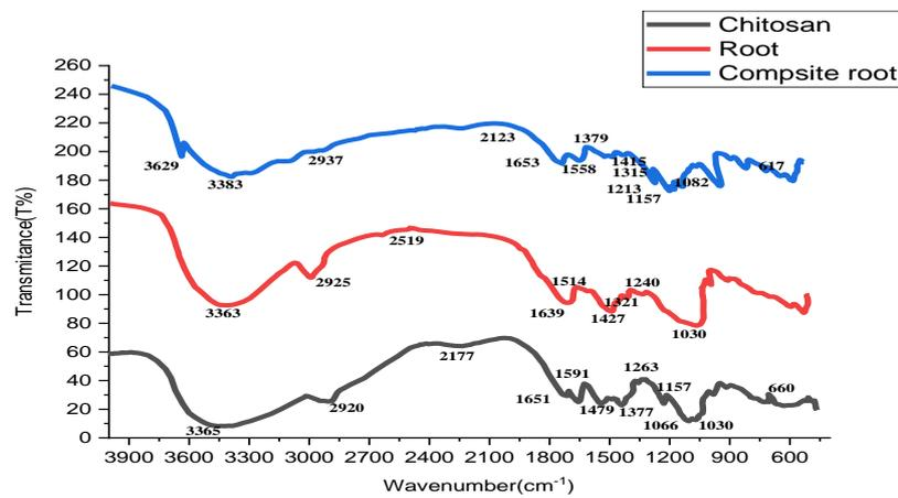
Figure 5. FTIR spectra of : (A) Chitosan beads; (B) Root powder hyacinth plant and (C) Chitosan beads with root powder hyacinth plant.
