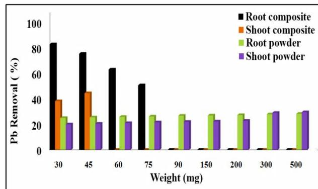
Figure 2. Removal percentage of Pb in the presence of water hyacinth parts within 24 hr and reference (0.0162 ppm)
