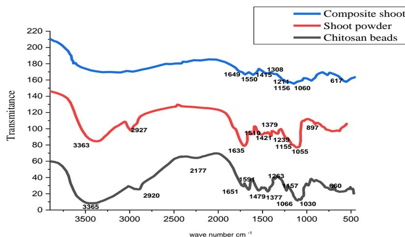
Figure 6. FTIR spectra of : (A) Chitosan beads; (B) Shoot powder hyacinth plant and (C) Chitosan beads with shoot powder hyacinth plant.
