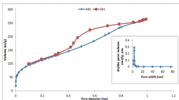
Figure 3. The N<sub>2</sub> adsorption-desorption for RHACI.
