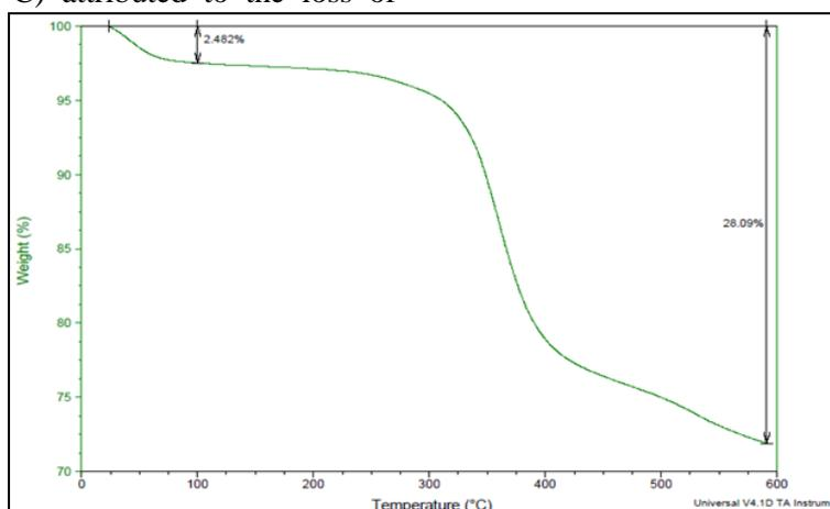
Figure 7. The thermal analysis TGA of RHACI.
