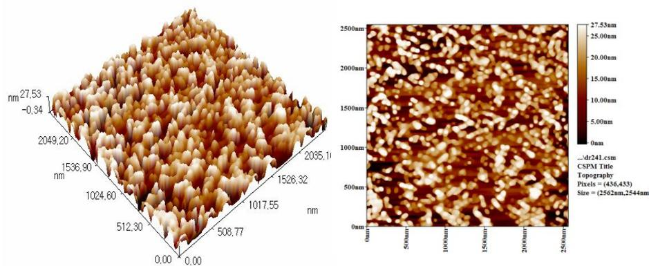
Figure 5. Three-dimensional AFM images for RHACI.
