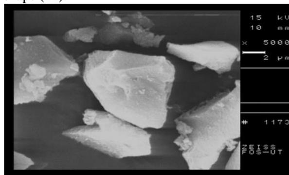
Figure 4. The SEM micrograph of RHACI powder.
