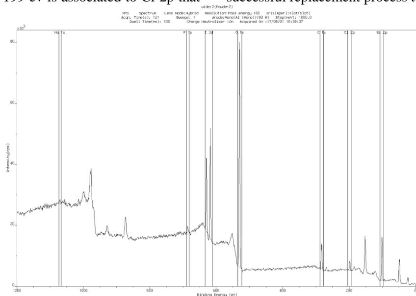
Figure 8. XPS spectrum of RHACI the C, O, Si, Cl and I content shown
