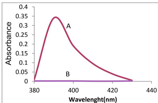
**Figure 2. Absorption spectra of (A) - 12 $\mu$ g/ml of thiaminehydrochloride with vanillin against reagent blank. (B) -reagent blank against water.**
