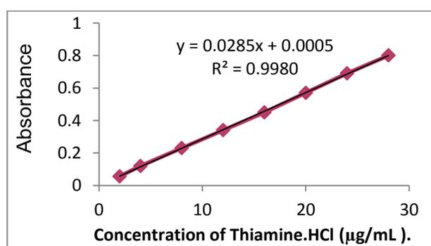
**Figure 5. Calibration curve of Thiamine hydrochloride**
