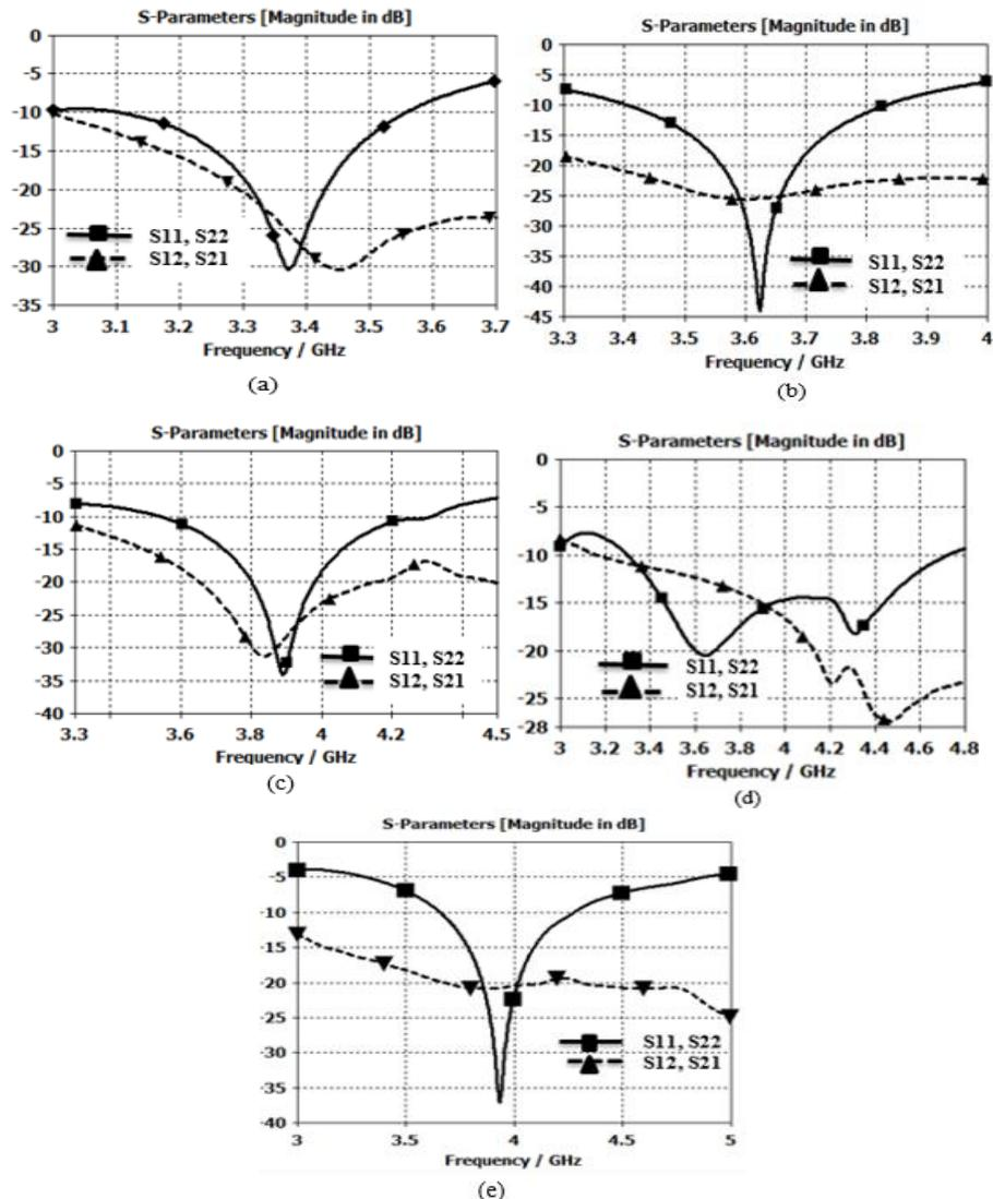
**Figure 2. Simulated Reflection Coefficients and Transmission Coefficients of the Two Antennas with LS1 and LS2 Slots. (a) S- Parameters of the (3.1-3.55) GHz Band, (b) S- Parameters of the (3.4-3.8) GHz Band, (c) S- Parameters of the (3.6-4.2) GHz Band, (d) S- Parameters of the (3.4-4.7) GHz Band, and (e) S- Parameters of the (3.7-4.2) GHz Band.**
