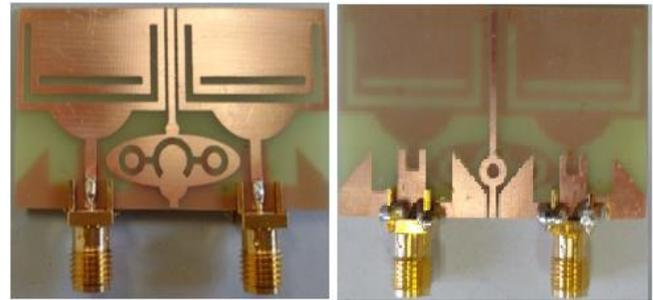
Figure 5. A photograph of the two fabricated antennas.
