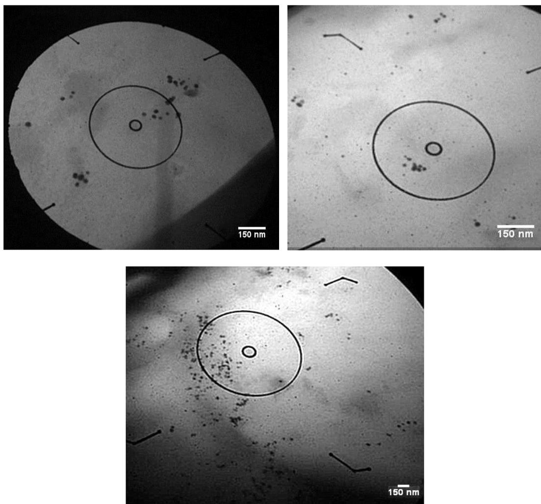
Figure 3. TEM images of GNPs synthesized using Al with GA .Size particle is 12- 17.5 nm (scale bar is 150nm)
