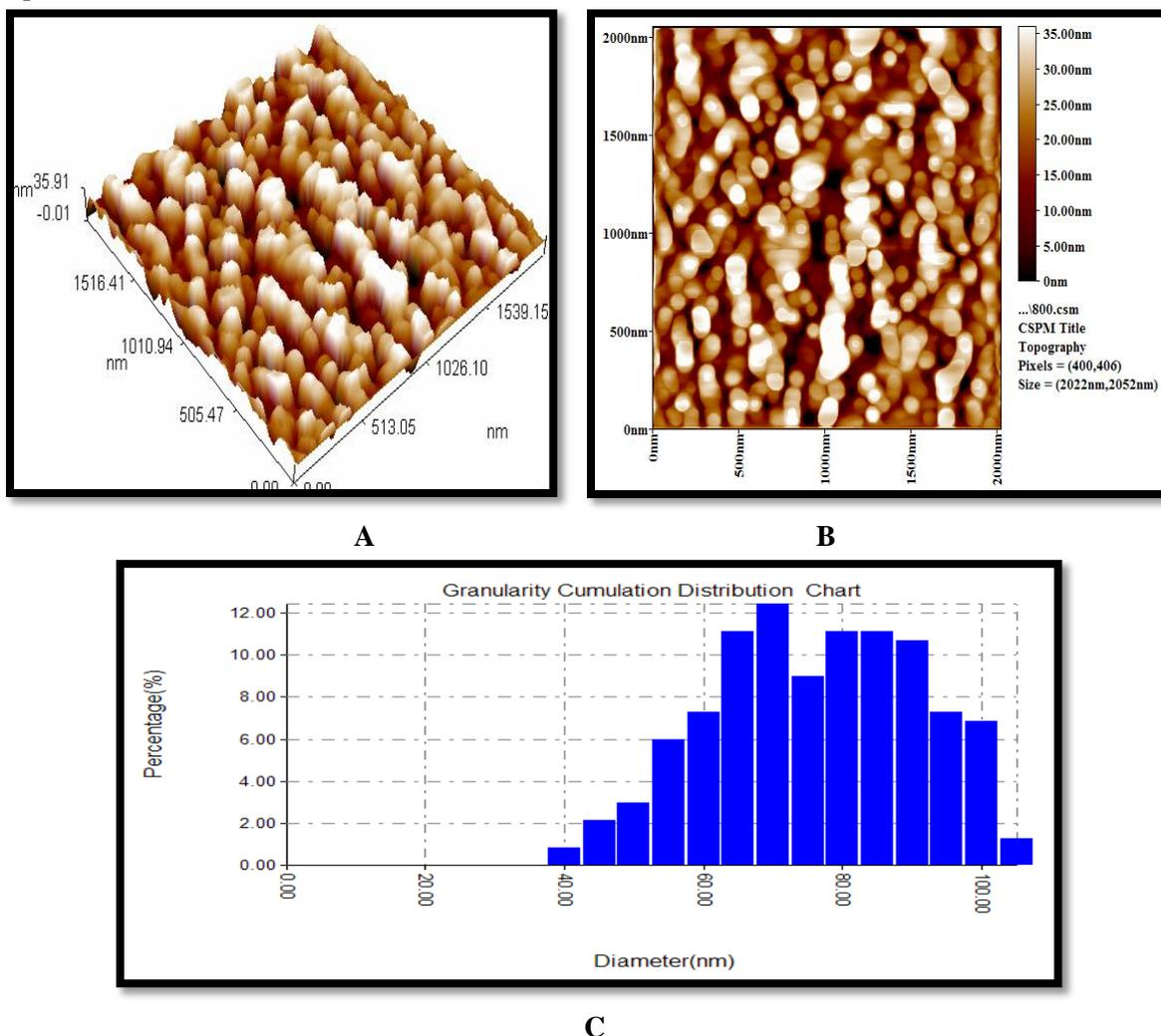
**Figure 2. AFM image of GNP<sub>s</sub> (A) 2D, (B) 3D, (C) Average particle distribution for GNP<sub>s</sub> 73nm. By using Al as reducing agent with gum Arabic as stabilizer**
