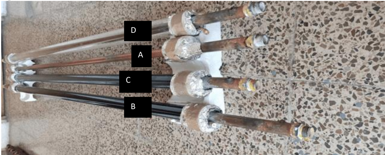
Figure 5. Types of receivers used in the study. (A) Copper tube surrounded by air. (B) Copper tube surrounded by aluminum fiber, black chrome-coated glass, and vacuum. (C) Copper tube surrounded by phase change material and black chrome-coated glass. (D) Copper tube coated by transparent white vacuum-sealed glass.
