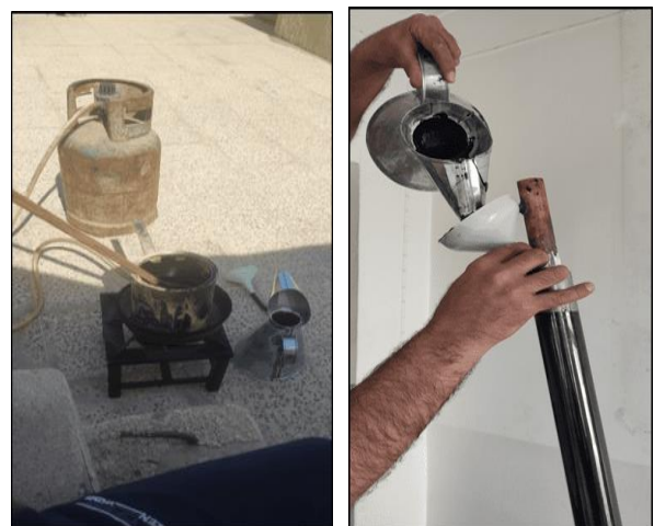
Figure 4. Primary materials for the copper tube surrounded by phase change material and black chrome-coated glass.
