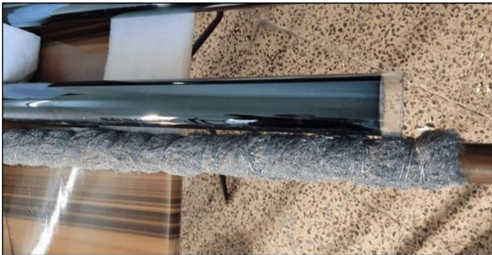
Figure 3. Primary materials for the copper tube surrounded by aluminum fiber and black chrome-coated glass.
