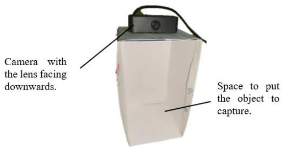
Figure 2. Proposed Image acquisition device
