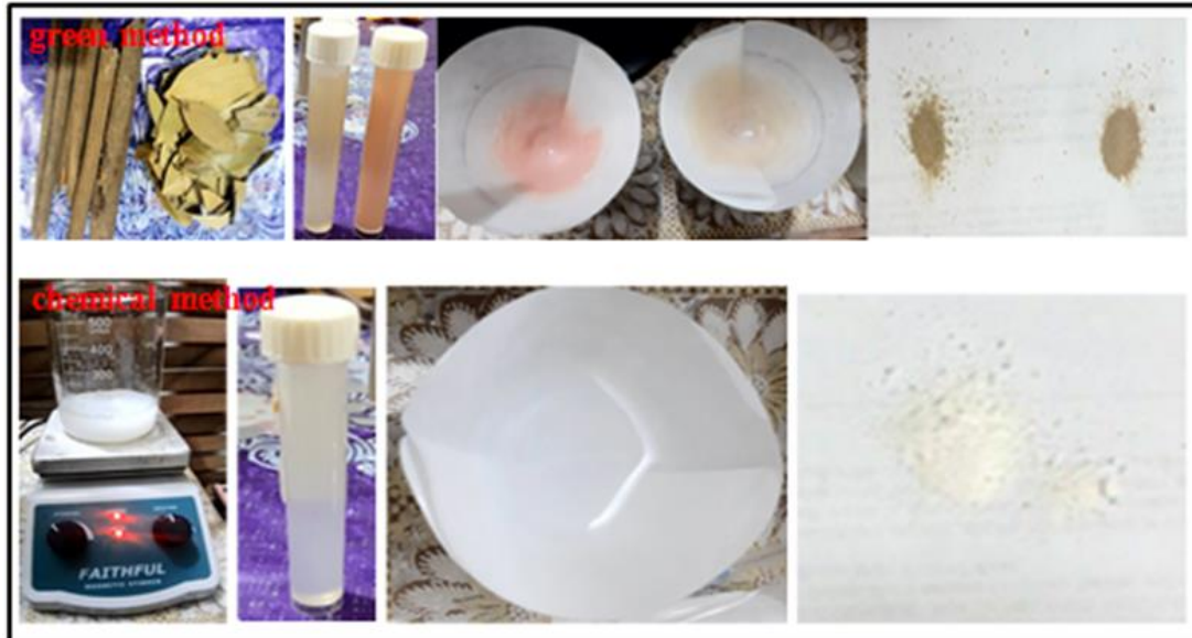
Figure 1. Process steps for preparing ZnO NPs by chemical and green methods.
