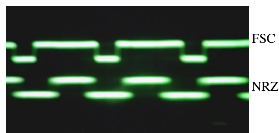
Fig.(4):the waveforms of NRZ and FSC signal with scale time set to 0.5 \mu s/div .
