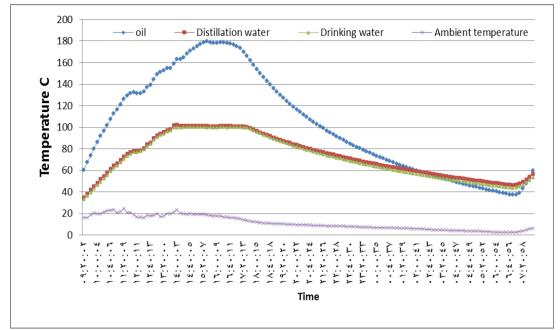
Fig (2)The comparison between temperatures of three receivers tubes and ambient temperature with time.
