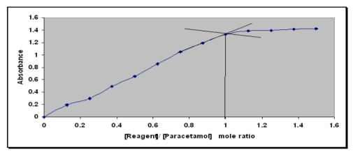
Fig. (3): Mole ratio of the azo dye of paracetamol with 2,4-di chloroaniline.
