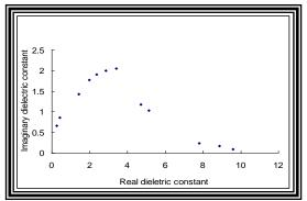
Fig (12): The relation between real and imaginary parts of dielectric constant.
