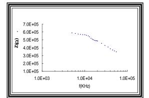
Fig (2): The frequency dependence of impedance at T=293K
