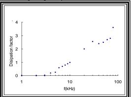
Fig (10): The frequency dependence of dissipation factor at temperature 313 K.
