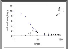
Fig (13): The frequency dependence of real and imaginary parts of dielectric constant.
