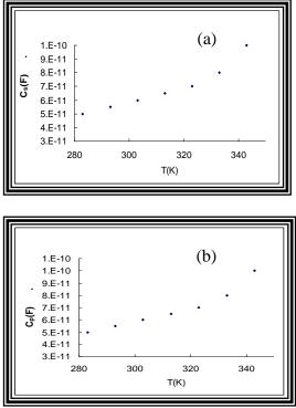
Fig (4): The The temperature dependence of a: series capacitance b: parallel capacitance
