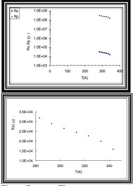
Fig (5): The temperature dependence of series and parallel resistance.
