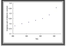
Fig (8): The temperature dependence of imaginary part of dielectric constant at a frequency of  $10^{3}$ Hz.
