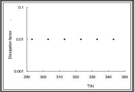
Fig (6): The temperature dependence of dissipation factor .
