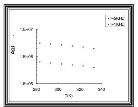
Fig (3): The temperaturedependence of impedance at f=1KHz and f=5KHz.
