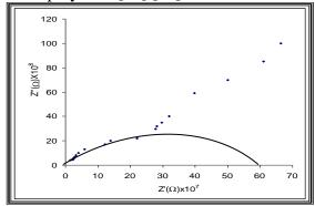
Fig (14): Cole-Cole plot for PPAB terminated by phenylenediamine doped with Na<sub>2</sub>[Fe(CN)<sub>5</sub>.NO].2H<sub>2</sub>O
