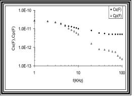
Fig (9): The frequency dependence of series and parallel capacitance at T=313 K.
