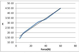
Figure 9. The Strain via Applied Force for 8mm Cell
