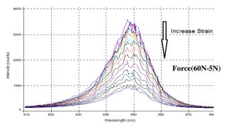
Figure 4. The Transmitted Spectrum of 5 mm Microbend Cell
