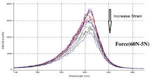
Figure 5. The Transmitted Spectrum of 8 mm **Microbend Cell.**
