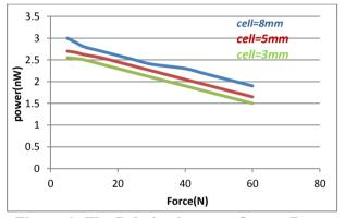
Figure 6. The Relation between Output Power and the Applied Force.
