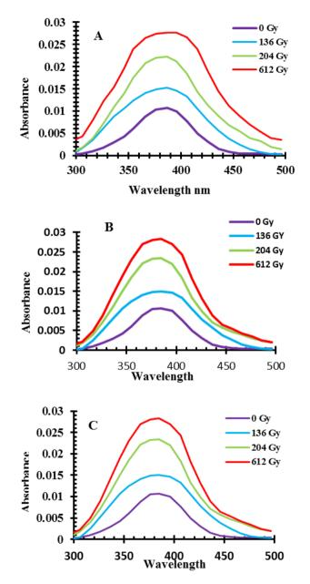
Figure.1 A, B and C: The C47 absorption spectra at different concentrations 10<sup>-4</sup>, 10<sup>-5</sup>, 10<sup>-6</sup>M at different doses 0,136,204 and 612 Gy.
