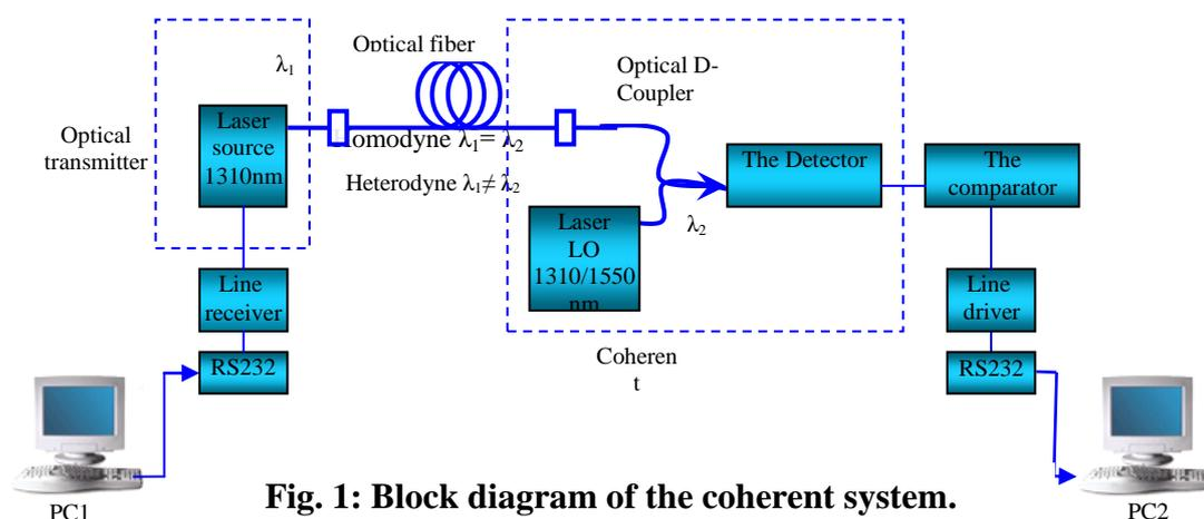
**Fig. 1: Block diagram of the coherent system.**
