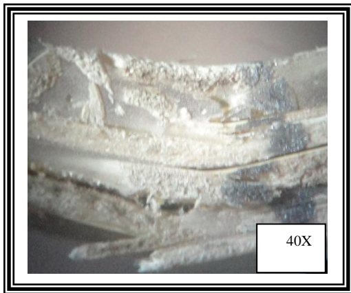
Fig. (14) photographic image for fracture regions shows the pull out of fiber after fracture for reeds \ polyester composite sample.
