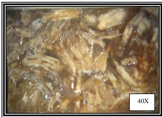
Fig. (9) photographic image for fracture regions of sawdust composite.
