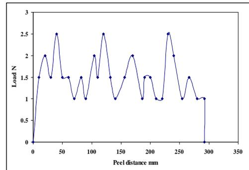
**Fig (6): Load – peel distanced curve for wet Al/PE. Crosshead speed (100 mm/min)**
