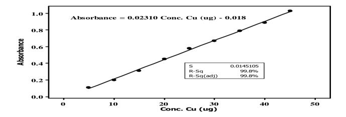
Fig (5) Calibration plot of Cu(II) DCH-18-Crowm-6
