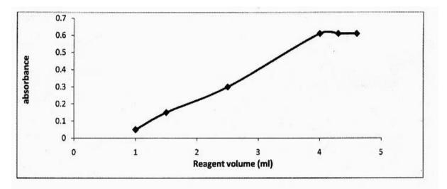
Fig (4) Effect reagent volume on the Extraction of Cu(II)
