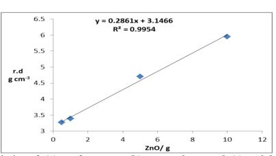
Fig (4) Variation of (a) surface area, (b) pore volume and (c) real density with ZnO additions for modified exposed to 500 °C
