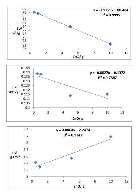
Fig(3): Variation of (a) surface area, (b) pore volume and (c) real density with ZnO additions
