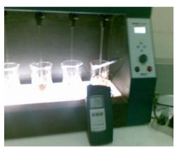
Fig. (1) Laboratory adsorption unit (Jar Test).
