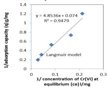
Fig. (6) Langmuir Isotherm adsorption model.
