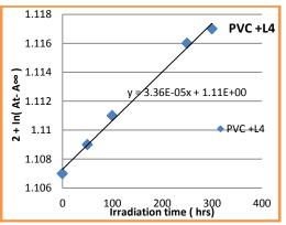
Fig. 5: In  $(At-A\infty)$  with Irradiation Time of PL4 for Modified PVC Chips
