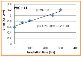
Fig. 2: In  $(At-A\infty)$  with Irradiation Time of PL1 for Modified PVC Chips
