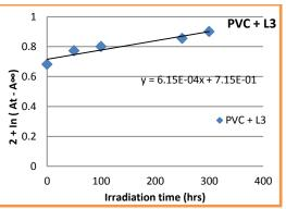
Fig. 4: In  $(At-A\infty)$  with Irradiation Time of PL3 for Modified PVC Chips
