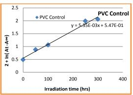
Fig. 1: In  $(At-A\infty)$  with Irradiation Time of PVC Control Chips
