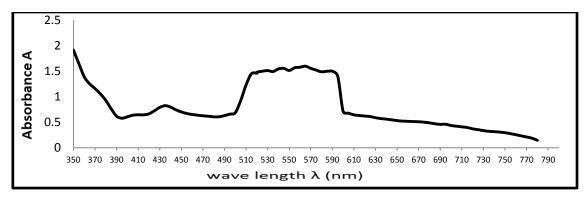
Fig. (2):Molecular Spectrum of KMnO<sub>4</sub>in Alkaline Medium.
