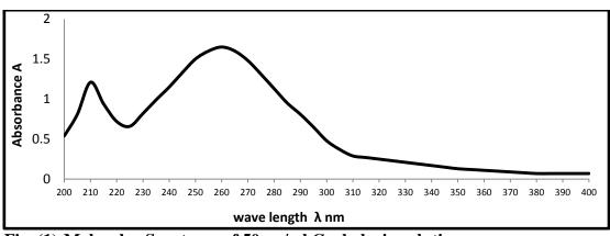
Fig. (1):Molecular Spectrum of 50 µg/ml Cephalexin solution.
