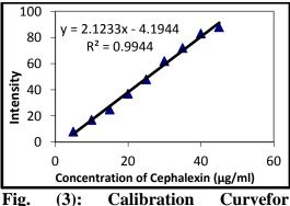
Cephalexin with  $KMnO_4$ in Alkaline Medium by Flame Atomic Emission Photometry.
