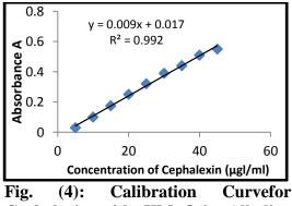
Cephalexin with  $KMnO_4$ in Alkaline Medium by Molecular Absorption Spectrophotometry.
