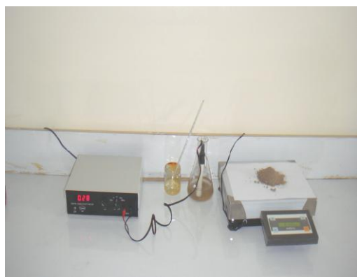
Fig.1 Shows the EC digital measurement device and the digital balance used in laboratory soil extraction EC test.
