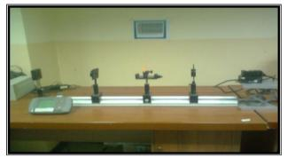
Figure 1. Z-scan setup
