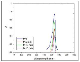
Figure 4. Shows the absorbance of the polymer model (PMMA) doping with Rhodamine (3GO) before and after exposure to plasma and for different times 5, 10, and 15 min.
