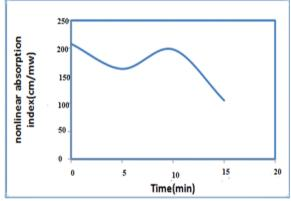
Figure 8. The relationship between the nonlinear absorption coefficient  $\beta$  and the time of the polymer membrane (PMMA) doping with Rhodamine (R3GO).
