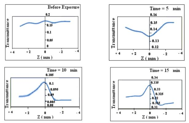
Figure 6. Shows (open-aperture Z-scan) curves of the polymer membrane (PMMA) doping with Rhodamine (R3GO) before and after exposure to plasma and for different times (5, 10 and 15) min.
