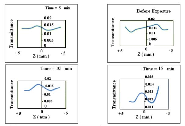
Figure 5. Shows the curves (closed-aperture Z-scan) of the polymer membrane (PMMA) doping with Rhodamine (R3GO) before and after exposure to plasma at different times (5, 10 and 15) min.
