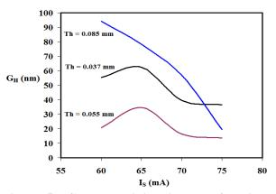
Figure 5. Copper grain's height as a function of sputtering currents for different values targets thickness.
