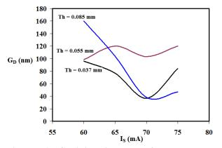
Figure 6. Grain's diameters of copper versus sputtering currents for different values of target thickness.
