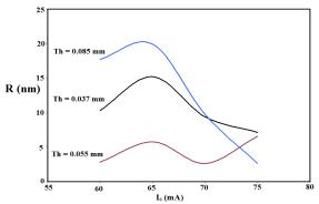
Figure 9. Roughness values versus sputtering currents for different values of target thickness.
