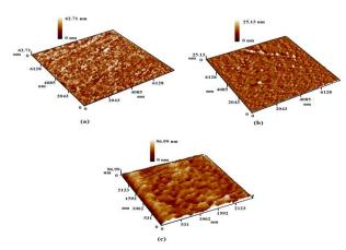
Figure 3. 3-D AFM images at sputtering current  $I_S = 70$  mA for different values of copper target thickness: (a) Th= 0.037 mm. (b) Th= 0.055 mm. (c) Th = 0.085 mm.
