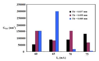
Figure 8. Maximum grain's size versus sputtering currents for different values of target thickness.
