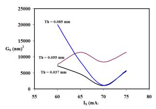
Figure 7. Average grain's size of copper versus sputtering currents for different values of target thickness.
