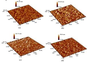
Figure 2. 3-D AFM images at copper target thickness 0.037 mm for different values of sputtering currents: (a)  $I_S = 60$  mA. (b)  $I_S = 65$  mA, (c)  $I_S = 70$  mA. (d) 75 mA.
