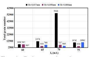
Figure 4. Total copper grain numbers versus sputtering currents for different values of targets thickness.
