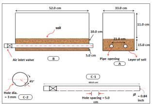
Figure.2 The dimensions of the stainless steel Bio pile system A: front view B: side view C-1: air supply tube C-2: cross section of air supply tube
