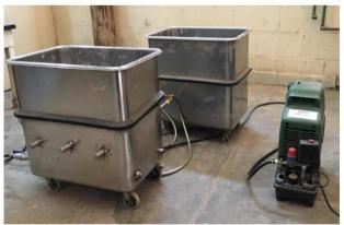
Figure.1The pilot-scale stainless steel tanks of Bio pile system
