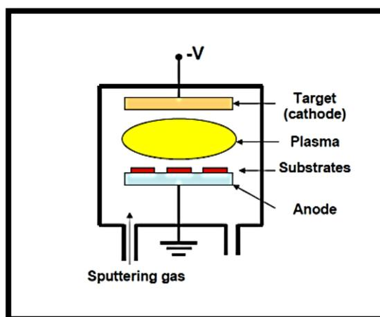
**Figure 2. Illustrate sputtering process.**
