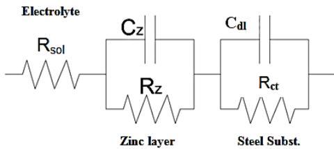
**Figure 7. Equivalent Circuit diagram, model: R (CR) (CR) at G-S uncoated in 3.5% NaCl Solution at 298K.**
