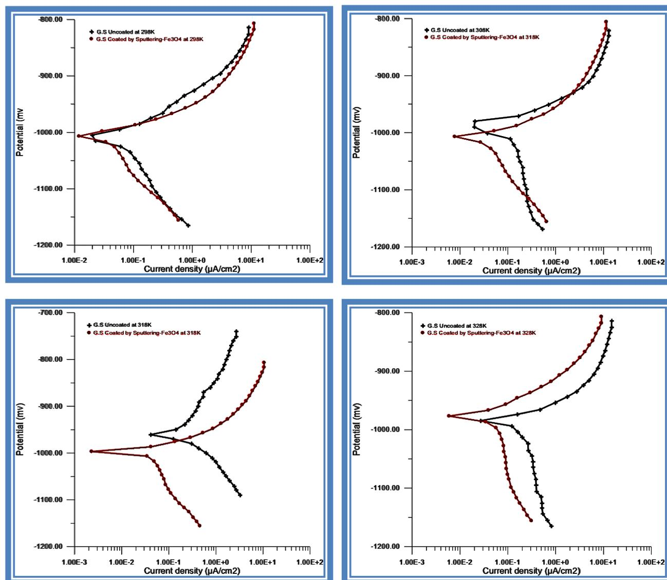
**Figure 4. Polarization curves for the corrosion of G-S Coated by the sputtering –Fe<sub>3</sub>O<sub>4</sub> at different temperature as compared with the polarization curves for Uncoated G.S.**
