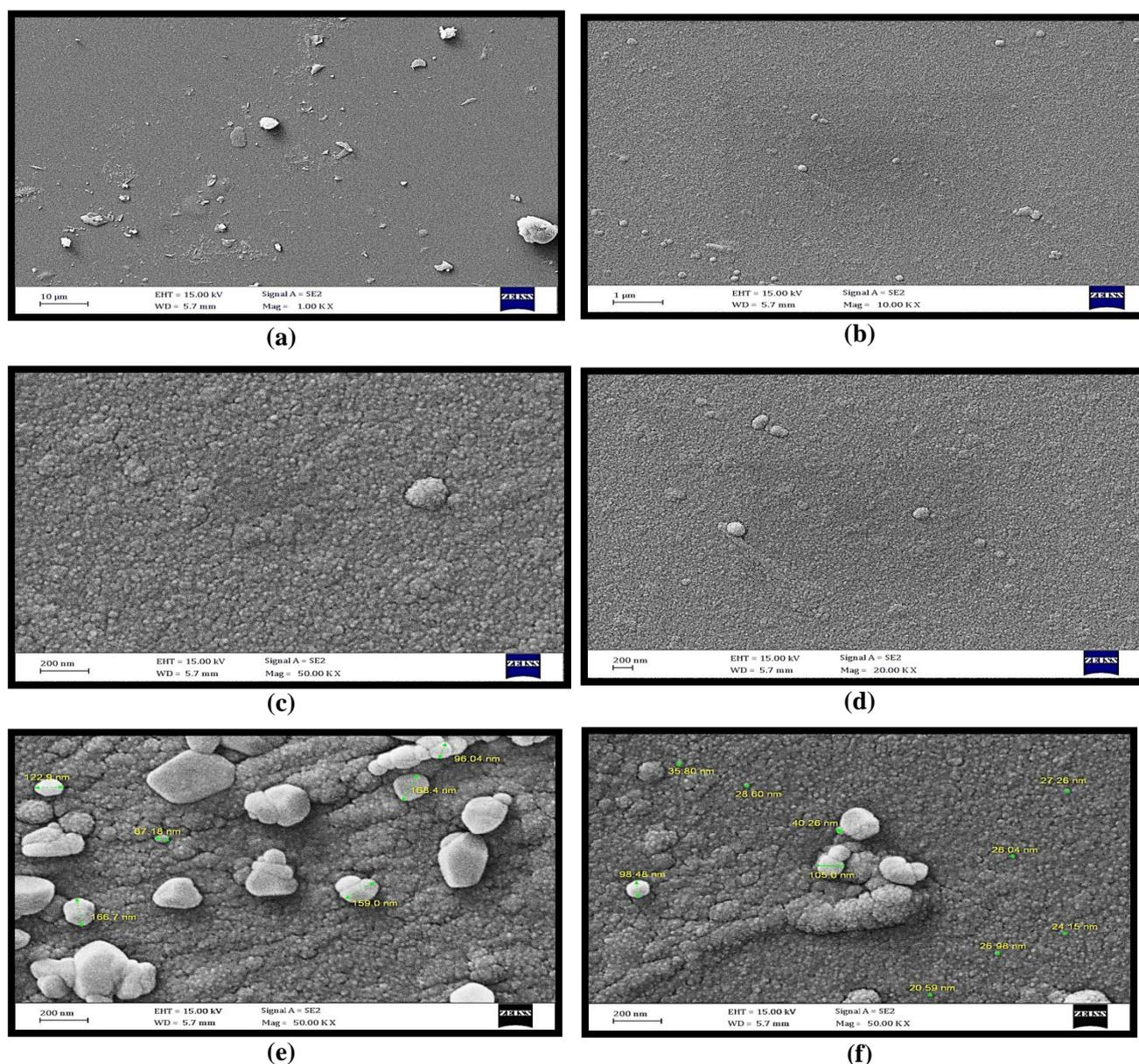
**Figure 11. SEM image of Magnetite  $Fe_3O_4$  coating (a/10 $\mu$ m), (b/1 $\mu$ m), (c/200nm), (d/200 nm), (e&f Particle Size).**
