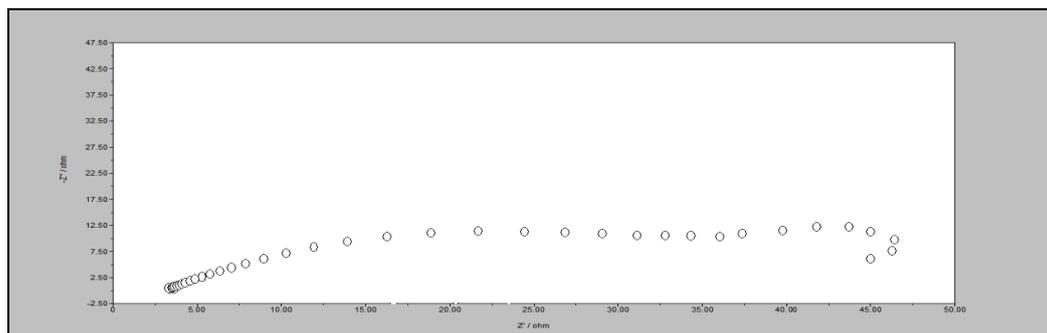
**Figure 5. Nyquist plot of the G-S uncoated in 3.5% NaCl solution at 298K.**
