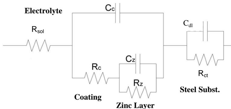
**Figure 10. Equivalent circuit diagram, Model R(C(R(CR))) (CR) for G.S Coated by  $Fe_3O_4$  in 3.5% NaCl Solution at 298K.**
