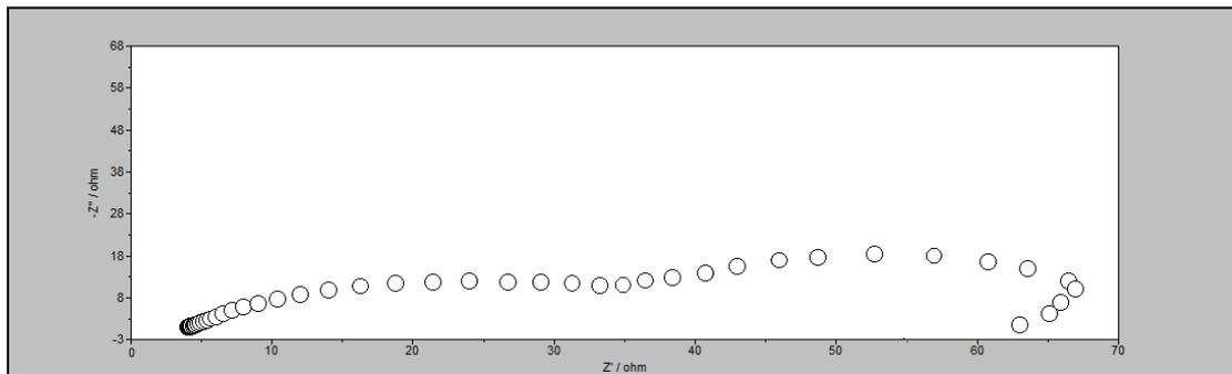
**Figure 8. Nyquist plot of G-S coated with  $Fe_3O_4$  by RF-Sputtering in 3.5% NaCl solution at 298K.**
