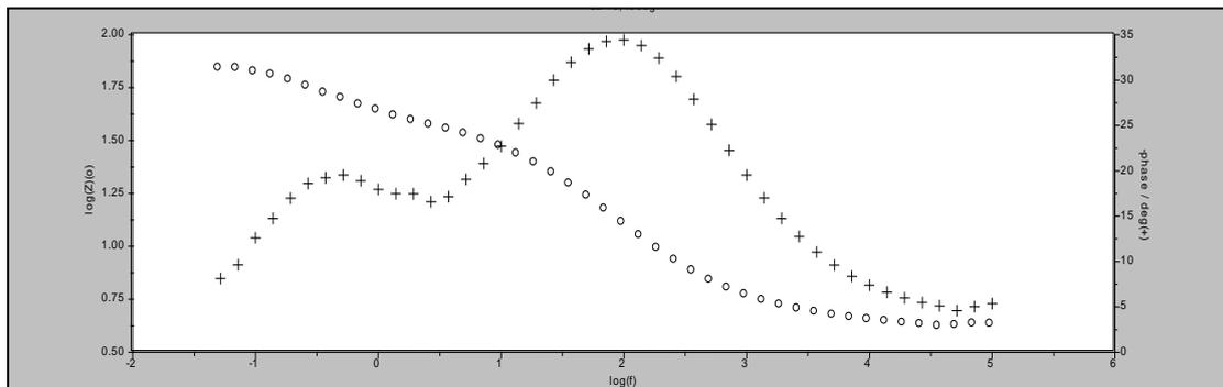
**Figure 9. Bode plot of the G-S Coated with  $Fe_3O_4$  by RF-Sputtering in 3.5% NaCl solution at 298K.**
