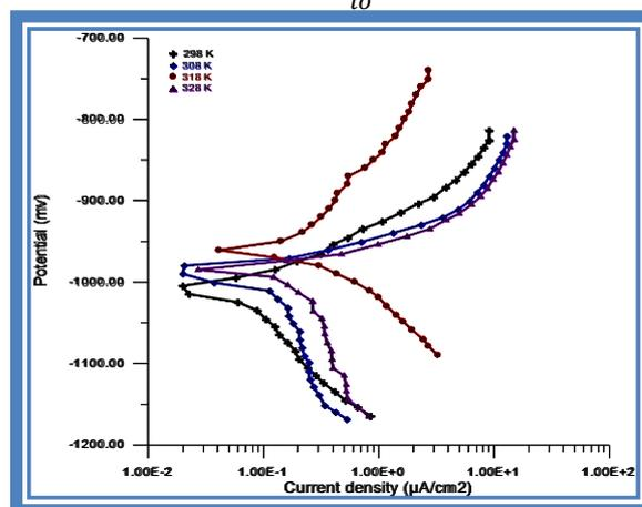
**Figure 3. Potentiostatic polarization curves for uncoated G-S in 3.5% NaCl solution at various temperatures.**
