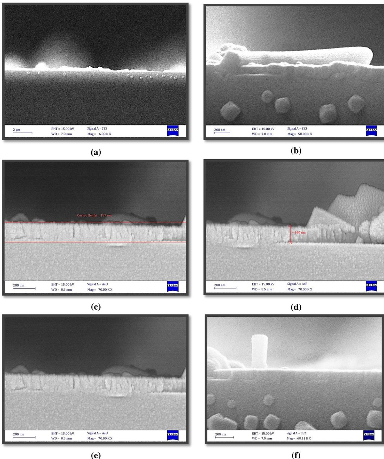
**Figure 12.** SEM images of Magnetite  $\text{Fe}_3\text{O}_4$  film .(a)2 $\mu\text{m}$ ), (b)200nm), (c) Cursor High = 187nm), (d) Cross Sectional outlook of Magnetite  $\text{Fe}_3\text{O}_4$  film coating indicate that thickness about 160 nm), (e&f 200 nm).
