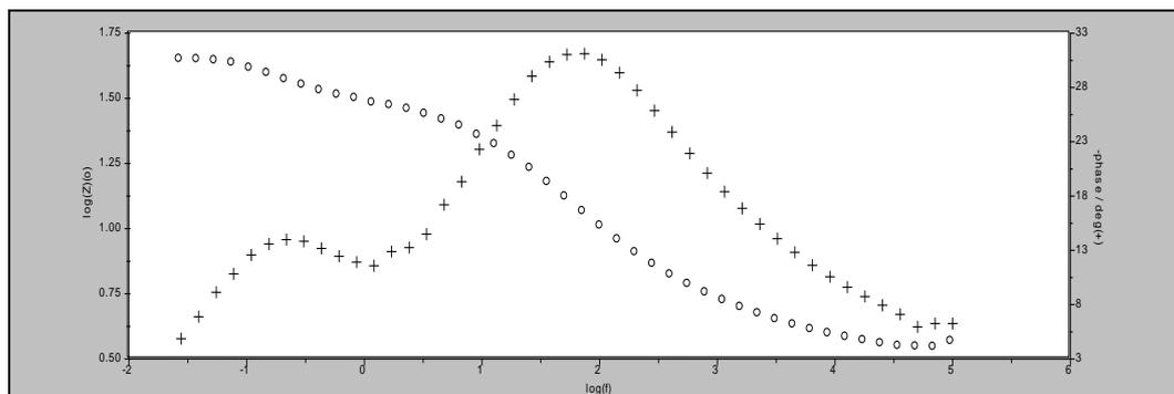
**Figure 6. Bode plot of G-S Uncoated in 3.5% NaCl solution at 298K.**
