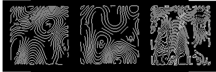
Figure 9. Applying Sobel edge detection on three frames of the HIP of Example 1
