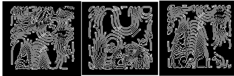
Figure 10. Applying Prewitt edge detection on three frames of the HIP of Example 1.
