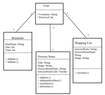
Figure 9. The class diagram of a mobile app for creating and managing grocery lists.
