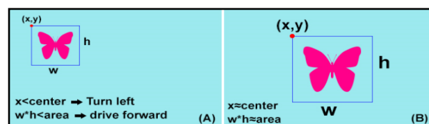
Figure 5. Steering modes: A) Object detected, B) Object tracked
