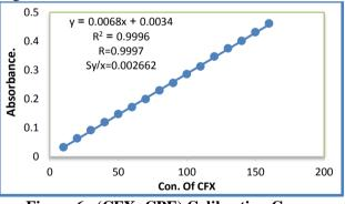
Figure 6. (CFX+CPE) Calibration Curve
