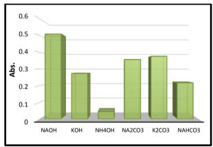
Figure 2. Data of absorbance for different bases with CFX
