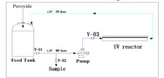
Figure 1. Schematic diagram of the H<sub>2</sub>O<sub>2</sub>/UV system
