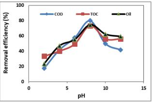
Figure 6. Effect of pH on removal efficiency of COD, TOC, and oil using O<sub>3</sub>/H<sub>2</sub>O<sub>2</sub>process.
