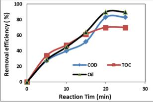
Figure 5 Effect of reaction time on removal efficiency of COD, TOC, and oil using  $O_3/H_2O_2$  process.
