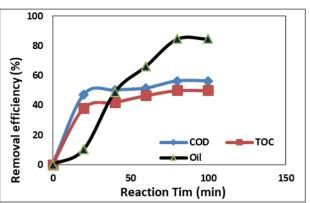
Figure 3. Effect of reaction time on removal efficiency of COD, TOC, and oil  $usingH_2O_2/UV$  process. Effect of pH
