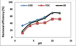
Figure 4. Effect of pH on removal efficiency of COD, TOC, and oil using H<sub>2</sub>O<sub>2</sub>/UV process.
