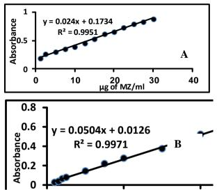
Figure 2.Calibration graphs for MZ determination (method A & B)
