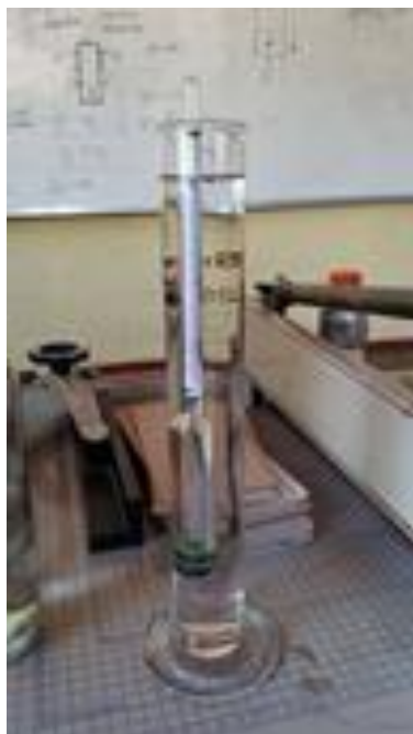
Figure 4. Concentration of ethanol determination using the hydrometer.
